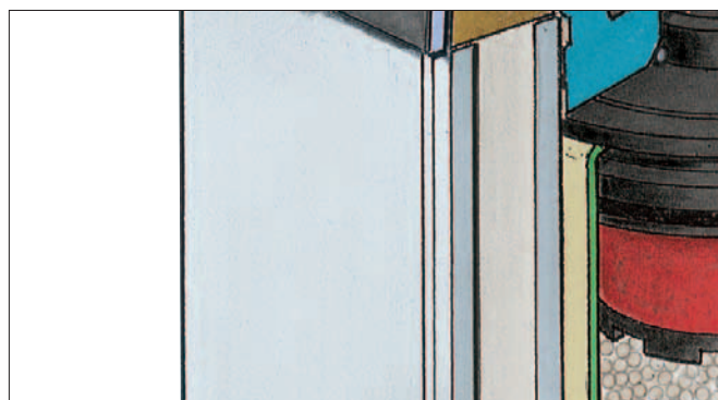
Corrosion protected by alocrom and epoxy painting.
